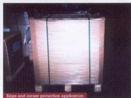
Edge and corner protection application
